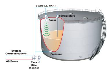
Example tank gauging system using the 4590 Tank Side Monitor and 4532/4539 Average Temperature Converter
