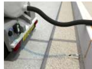
The truck mounted grounding system, the Earth-Rite MGV, tests grounding points to ensure they are capable of grounding trucks.
