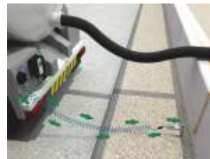
Continuous Ground Loop Monitoring check
